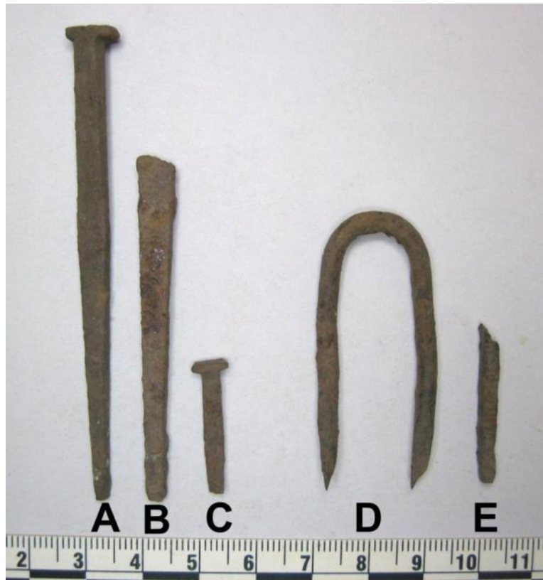
Plate 34: Metal artifacts from BbGd-60, TS3 1x1 unit – A-C) machine cut nails, D) fence staple, E) wrought nail
