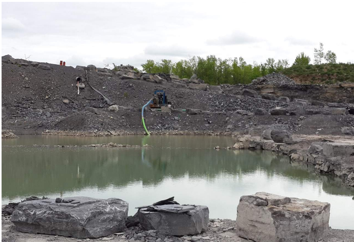
Photo 10: Wash plant pond with pump for flood events
